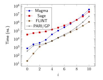
We present some timings for arithmetic in  $\mathbb{Q}_q \mod p^N$  where p = 17,  $N = 2^i$ , i = 0, ..., 10, comparing the three systems Magma (V2.19-2), Sage (current github, 5.12.beta4) and FLINT (current github) on a machine with Intel Core i7-2620M CPU running at 2.70GHz.
